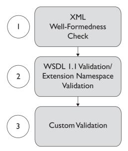
Figure 14.14 The Three Stages of WSDL Validation
