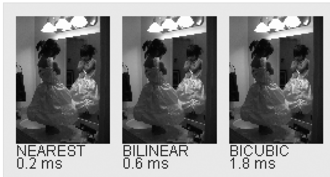
Figure 4-10 Close-up of the NEAREST , BILINEAR , and BICUBIC scaling results. All have similar artifacts for this large downscale.
