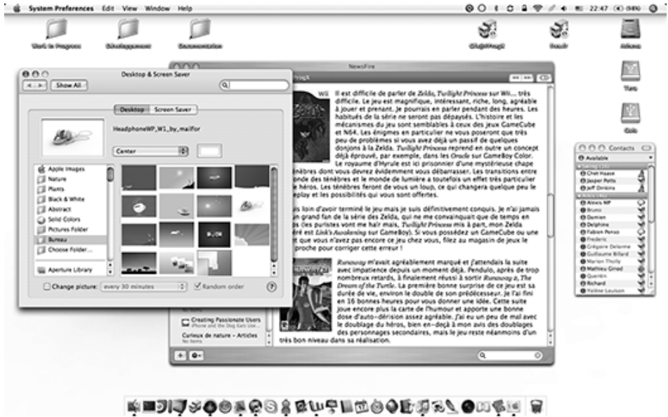
Figure 16-13 The focused window has a stronger drop shadow to make it stand out.
