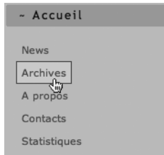
Figure 16-18 This Web page changes the background and the border of the highlighted item.
