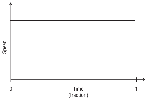
Figure 14-4 Default animation behavior, with no acceleration or deceleration: The speed of animation is constant.
